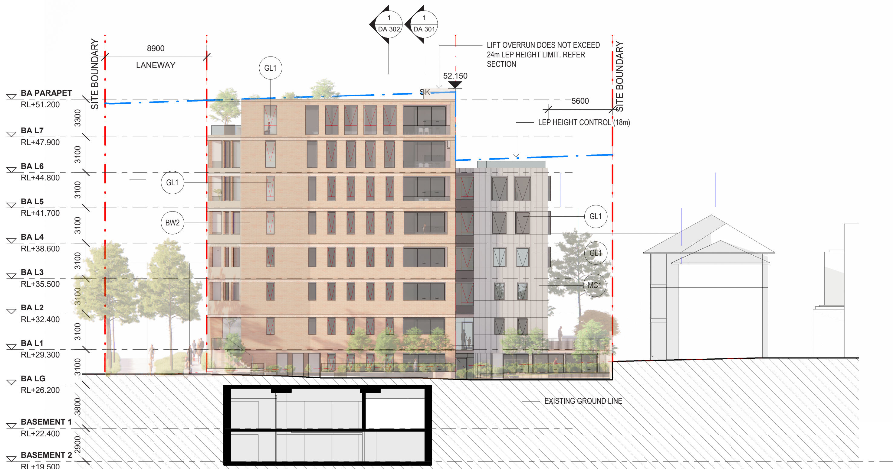
1 WESTERN ELEVATION - BUILDING A 1 : 200
